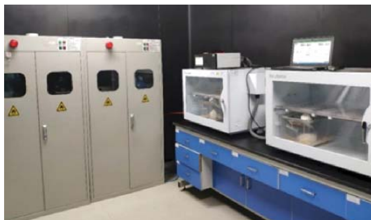
Figure 1 Attendor animal gas control system and oxygen box, with animals in the box
