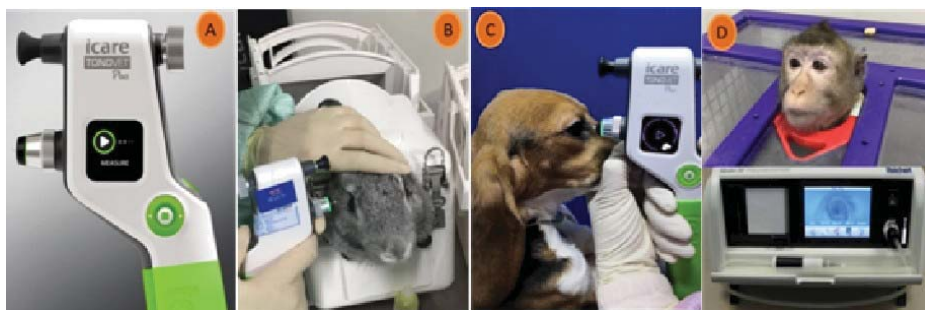
Figure 1. Rebound tonometer and the measurement of intraocular pressure of conscious rabbits, dogs and monkeys
